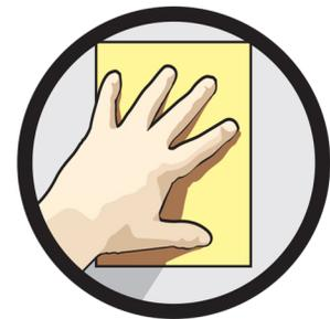
3. Remove film backing on other side of application and expose to UV or sunlight. Curing times depend on UV intensity between 5 minutes (sunny) and 50 minutes (cloudy) or use a UV light indoors with a minimum of 51 lumens.
