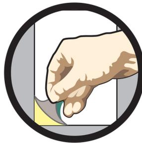
2. Remove white backing tape to expose the sticky resin. Apply patch to repair area with sticky side down and press firmly.
